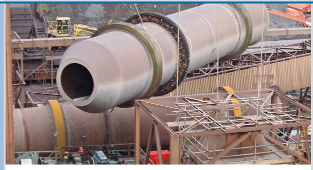
Sludge, especially that derived from mining operations, is granulated in a continuous process comprising two consecutive and continuous steps in which the sludge is mixed and granulated in the CEMTEC mixing/granulating drum.
